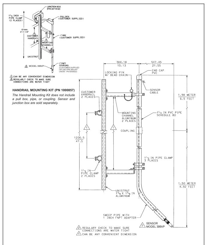
FIGURE 2-6. SENSOR SHOWN IN HANDRAIL MOUNTING ASSEMBLY (PN 11275-01)
